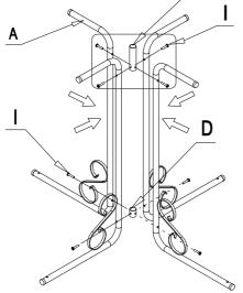
Screw 4 Casters on to the base of Leg Stands, and secure with Screws as shown.
