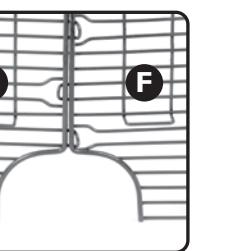
Place the Front Wire Panel w/ Door (E) so the spring loaded door latch opens downward. Place the Back Wire Panel (F) so that the opening for the bottle nozzle is on the bottom. Connect the Front Wire Panel w/ Door (E) to the Back Wire Panel (F) by hooking the wire into each other (as pictured).
