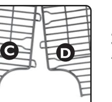
Place the Front Wire Panel w/ Door (C) so the spring loaded door latch opens downward. Place the Back Wire Panel (D) so that the opening for the bottle nozzle is on the bottom. Connect the Front Wire Panel w/ Door (C) to the Back Wire Panel (D) by hooking the wire into each other (as pictured).
