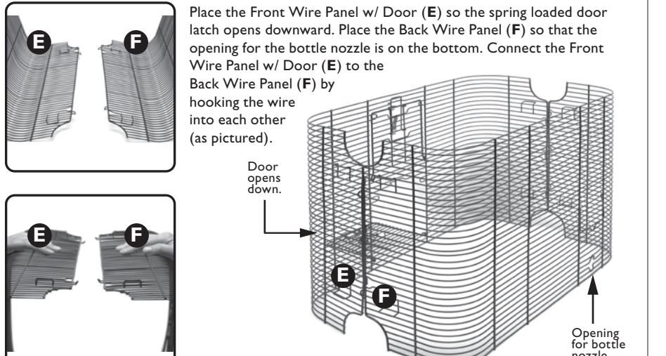
Place the Front Wire Panel w/ Door (E) so the spring loaded door latch opens downward. Place the Back Wire Panel (F) so that the opening for the bottle nozzle is on the bottom. Connect the Front Wire Panel w/ Door (E) to the Back Wire Panel (F) by hooking the wire into each other (as pictured).
